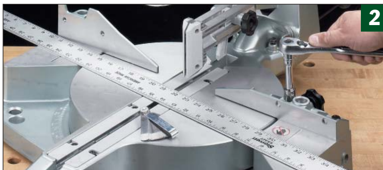
▲ Hitachi's two-piece fence lets you adjust both faces independently and make them perfectly parallel to
