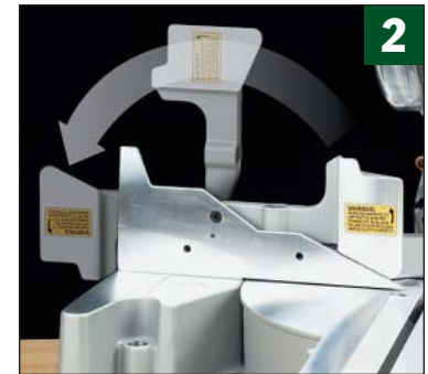
▲ Extending the subfence or moving it to allow the saw to bevel all the way to the left is a simple matter of flipping it out of the way.
