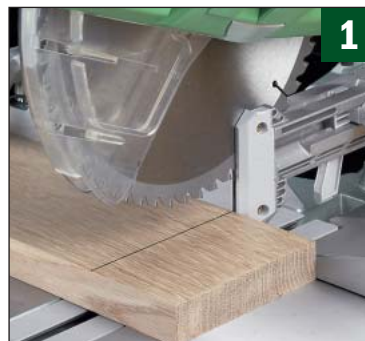
▲ Hitachi's saw features a "guard" that serves as an accurate alignment device. The kerf in the guard is cut during the initial setup.
