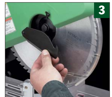
▲ Blade changing on the Hitachi is easy thanks to a cover that offers quick access to the arbor.
