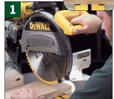
▲ The handle and trigger are easy to use with either hand. Slots in the blade guard provide a clear view of the intended cut line (Detail a).
