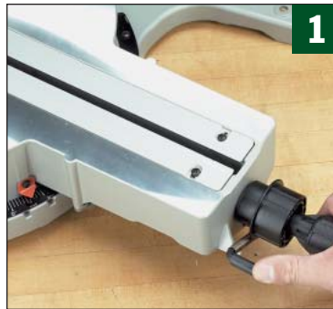
▲ Makita made their saw user friendly with easy operating controls for the detent override (the lever) and rail lock (the thick collar).
