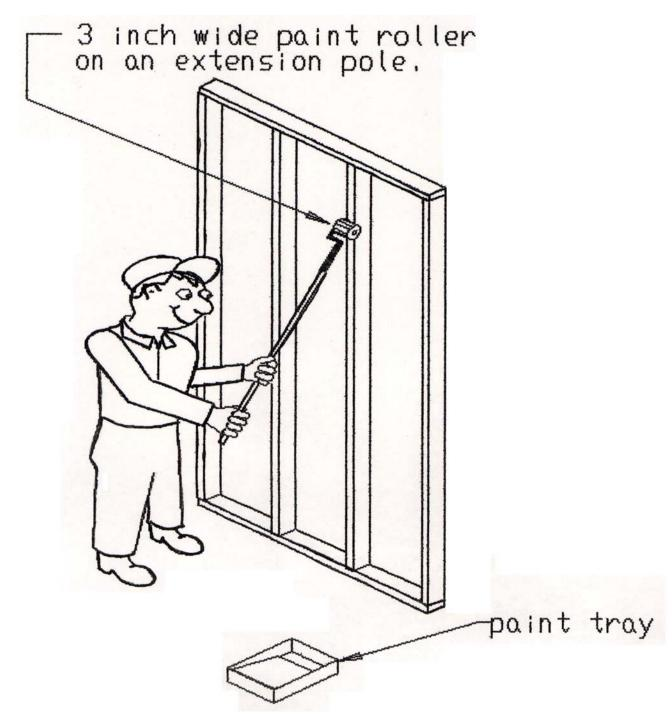
Roll on Regal Wall warm weather or cold weather adhesive over fabric to each stud face. Use a 3-inch wide *maximum* paint roller to cover. Use a handle extension for easy reach. A paint tray (recommend plastic) can be used for the adhesive. 1-coat is sufficient. Allow adhesive to dry before installing cellulose insulation. Drying time dependant upon room temperature.
