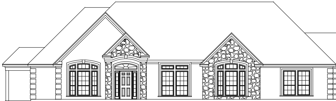
FRONT ELEVATION / STUCCO AND STONE / SCALE 1/4" = 1'
