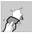
b. Apply a skim coat of joint compound with a joint-finishing knife to damaged area and feather to get a smooth finish. Let dry and apply second coat if necessary. Sand and prime when dry.
