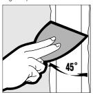
To apply joint compound neatly, dip the knife sideways into the pan so you load only half the width of the blade. For best results, joint compound should be thinned slightly with water for easier application. Add water in small increments (for one gallon of compound, add water in 2 oz. increments).
