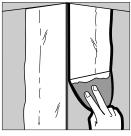
Use an 8" or larger finishing knife for outside corners (4"-6" knife for inside corners) to apply a finishing coat of the same ready-mixed or setting-type compound. Feather compound 8" (200 mm) from nose of trim for outside corners (1" [25 mm] past previous coat for inside corners). Let dry. Sand and prime.
