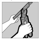
Force bead onto corner being careful that the flanges don't spread beyond 90° angle, making it hard to cover them with joint compound.
