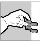
c. Measure and cut new drywall panel section to fit damaged area. Screw through new drywall into each drywall repair clip. Screw into drywall, positioning screw opposite screw holding clip and about 3/4" from edge.
