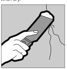
c. To repair a popped nail, drive and dimple new nail 1-1/2" from popped nail. Drive and dimple popped nail. Cover with joint compound. Sand and prime when dry.
