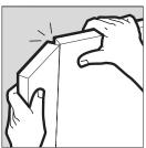
Use utility knife with sharp blade for scoring. Complete cutting by running knife through back paper for the length of the panel and snapping back to face.
