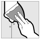
Center and lightly press tape into wet joint compound with fingers. Draw 5" knife firmly along joint to tightly embed tape. Be sure there is sufficient joint compound under tape to prevent blistering of the tape.
