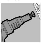
Use an electric screwgun equipped with an adjustable screw depth control head and Phillips bit. If an electric drill is used, be careful not to overdrive screws.
