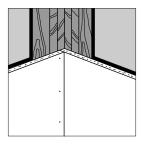
To join panels at an outside corner, lap the end of the second board over the end of the first. Make sure panels abut neatly—do not overlap or extend the end of the second board beyond the first. Fasten both panel ends to their common stud.
