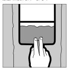
Apply a 7"-8" coat of joint compound to each side of butt joints and feather. Compound should extend beyond first coat for a total width of 14".
