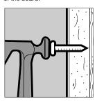
Double-nailing reduces the likelihood of nail pops. It is highly recommended for ceilings. Drive first nails 12" o.c. along framing in the field of the board and second nails about 2" from the first. Fasten the perimeter 7" o.c. for ceilings and 8" o.c. for walls.
