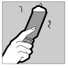
b. To repair a small hole or crack, trim any loose pieces from the damaged area and wipe it clean. Fill with joint compound, using a putty knife. Let harden. Add second coat if necessary. Sand and prime when dry.
