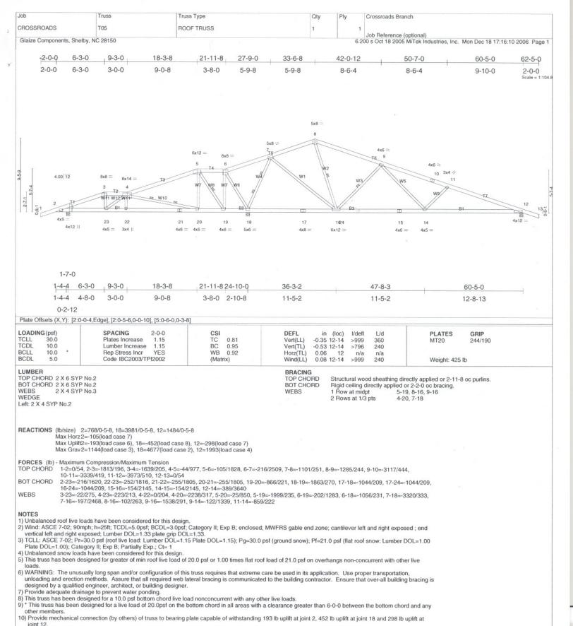
11) This truss is designed in accordance with the 2003 International Building Code section 2306.1 and referenced standard ANSI/TPI 1.
