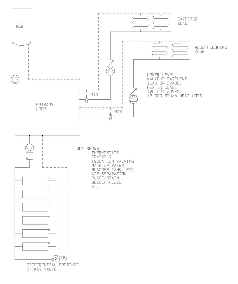
MAIN FLOOR, SIX (6) PANEL RADIATORS, ALL WITH TRVs, 41,000 BTL/h HEAT LOSS
