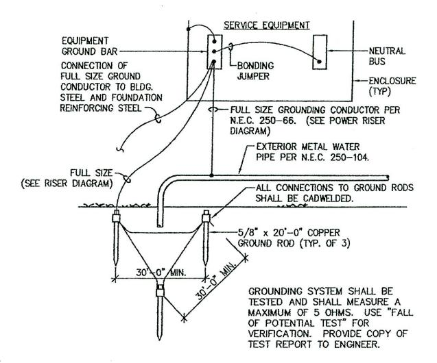
GROUNDING ELECTRODE CONDUCTOR DETAIL
