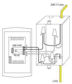
**WARNING:** Special CO/ALR solderless connectors must be used when connecting with aluminum conductors.
