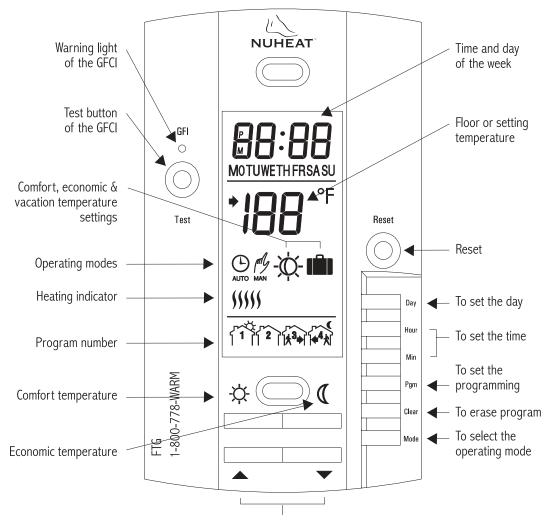
Up & down to adjust the temperature setting
