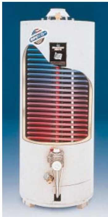
Figure 5. This flat plate heat exchanger (left) is adequate for heating a 4,000-square-foot house in the author's climate (75,000 Btu/hr.). Where code officials insist, the author uses a Combi-Cor unit (right), which has an internal coil exchanger. The coil's double wall offers secondary protection against contamination of the drinking water by the heating fluid.
