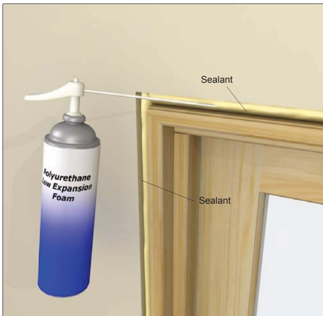
Figure 15 Apply low expansion foam between frame and rough opening.
