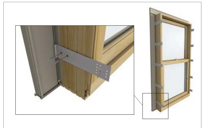
Figure 7 Apply brackets/clips to units with flat casing (if applicable).
