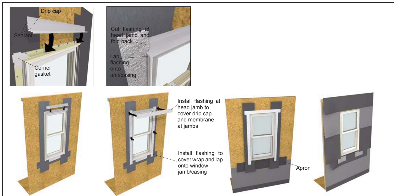
Figure 13 Sealing the installation in building paper applications.
