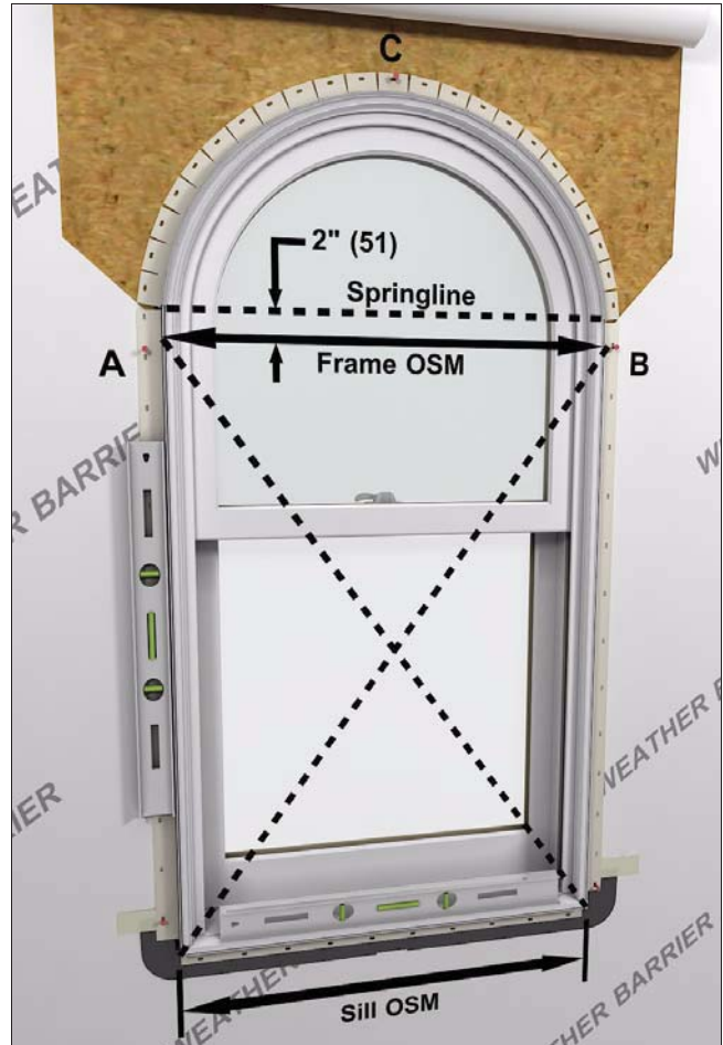
Figure 17 Shim and secure.
