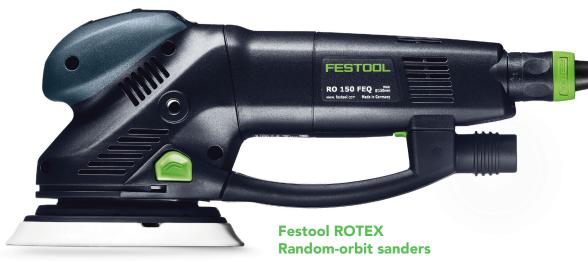
Festool ROTEX sanders are three state-of-the-art tools in one, switching instantly from rotary mode for fast material removal to the classic eccentric action for fine sanding and back to rotary for polishing with Festool polishes and polishing sponges. Festool's new MULTI-JETSTREAM 2 sanding pads are standard, collecting dust from more areas of the disk, including the edges, for better efficiency, cooler operation, and longer abrasive life.
