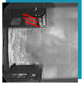
Figure 2. Cooking Plume Displaced by Short Circuit Supply Causing Hood to Spill.
