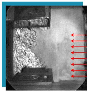
Figure 5. Effective Plume Capture When Makeup Air is Supplied at Low Velocity from Displacement Diffusers.
