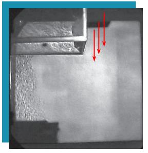
Figure 5. Effective Plume Capture with Makeup Air Supplied Through a 16-in wide Perforated Perimeter Supply.
