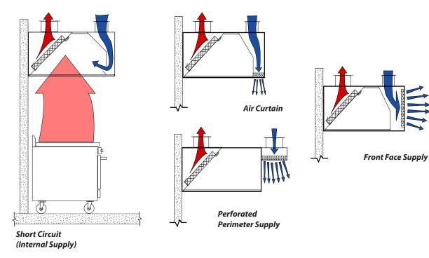
Figure 1. Types of Makeup Air Supply Integrated with the Hood.
