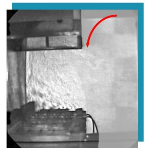
Figure 6. Thermal Plume Pulled Outside Hood by the Air Discharged from a 4-Way Diffuser.
