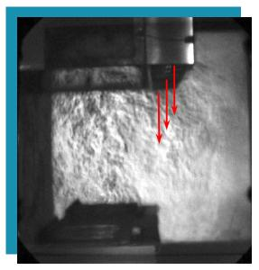
Figure 3. Cooking Plume Being Pulled Outside the Hood by the Air Curtain.
