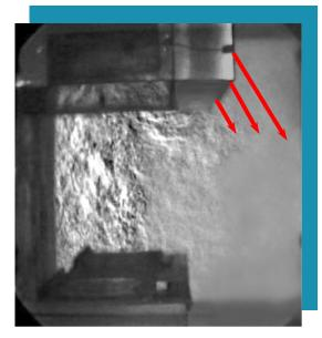
Figure 4. Cooking Plume Pulled Outside the Hood by a Poorly Engineered Front Face Supply.
