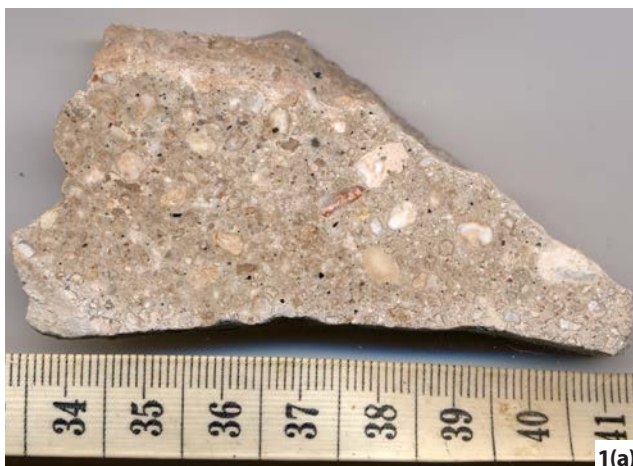
Figure 1: Samples of old gypsum plaster floors: (a) Typical colour and texture. (b) The varied composition found.
