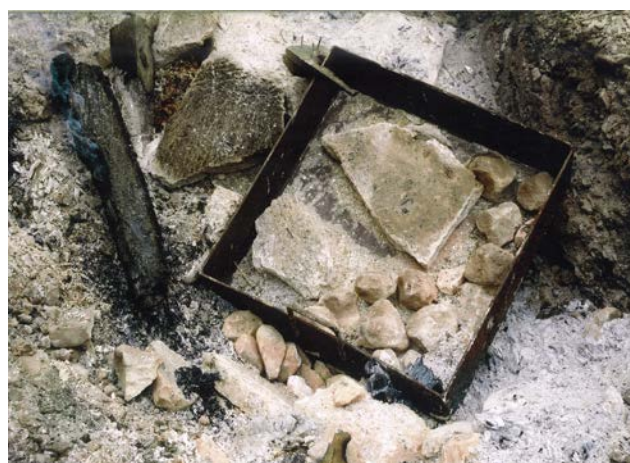
Figure 5: Trial gypsum-burning on an SPAB course.
